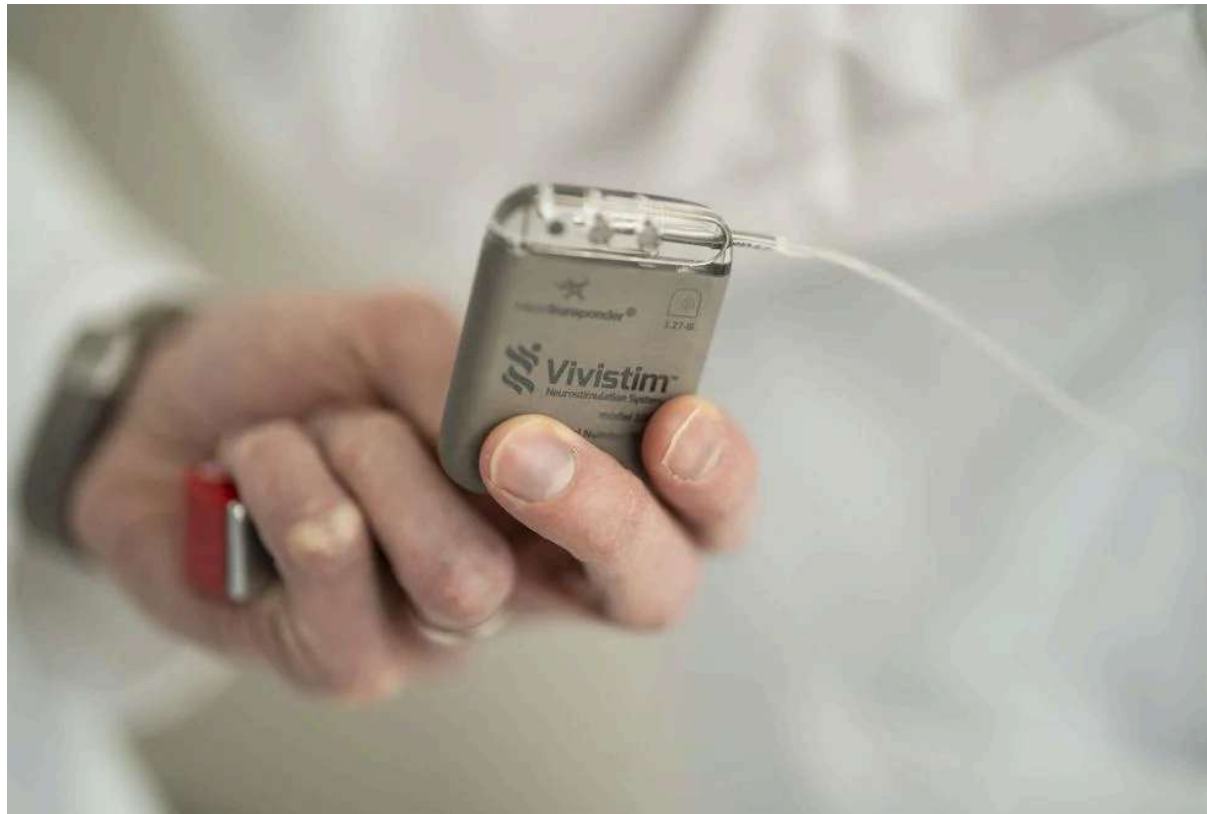
A Vivistim generator implant. The implant, programmed by clinicians and therapists, is placed in the chest and carries stimulation to the vagus nerve through a lead wire.
